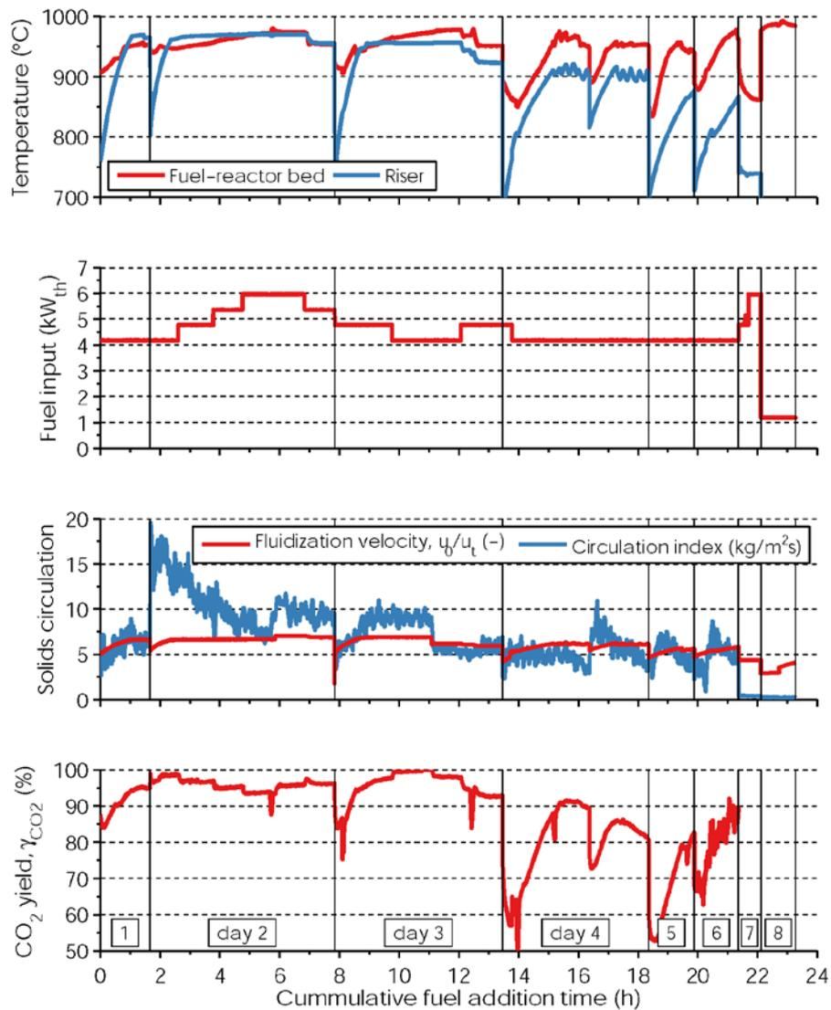
**Figure 5: Overview of the parameters varied (temperature, fuel input, solids circulation) and the performance of the process ( $\text{CO}_2$  yield,  $\gamma_{\text{CO}_2}$ ). The dimensionless fluidization velocity,  $u_0/u_t$ , was calculated with  $u_t = 0.43$  m/s.**
