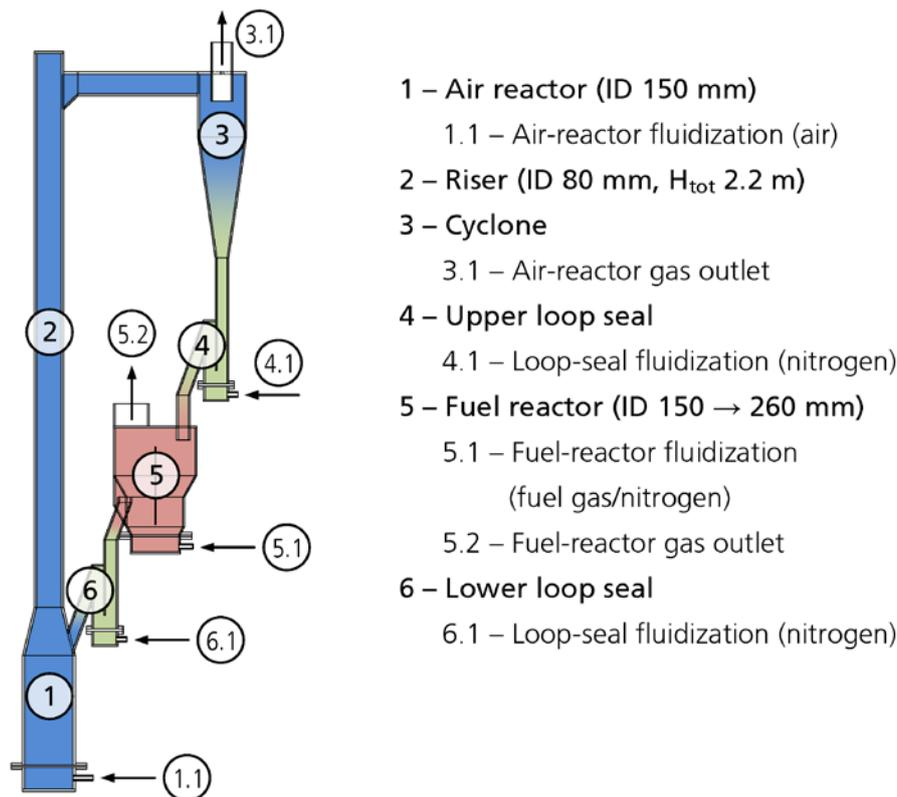
Figure 3: Schematic of the 10 kW chemical-looping combustion reactor
