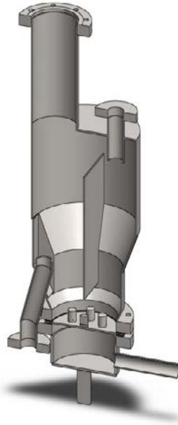
**Figure 4: 3D visualization of the fuel reactor with vertical separation wall between particle inlet and outlet.**
