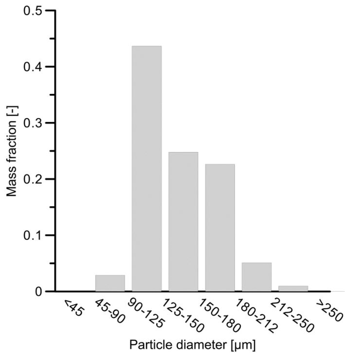
Figure 1. Fresh particle size distribution for the selected impregnated particles
