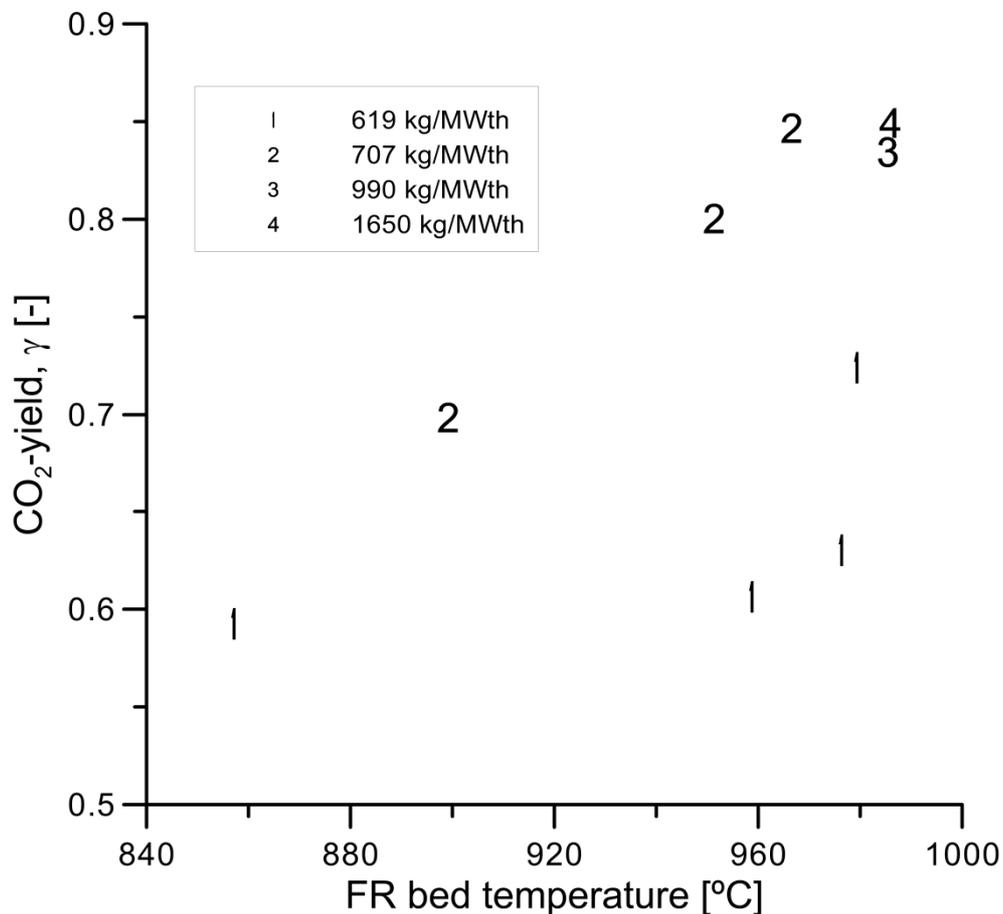
Figure 6. CO<sub>2</sub>-yield as a function of FR bed temperature and specific fuel reactor inventory.
