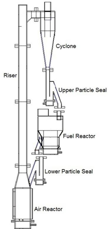
*Figure 3. A schematic picture of the 10 kW fluidized-bed reactor. Auxiliary equipment not shown.*
