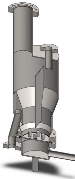
*Figure 4. A 3 dimensional image of the fuel reactor with the vertical plate.*
