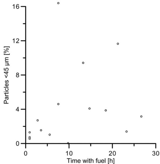
Figure 5. Fraction of fines in the elutriated material as a function of operating time.
